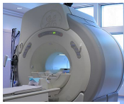
CRITICAL WARNING: AVOID METALS IN MRI Within the metallic cones of an MRI scanner, the patient is surrounded by two electromagnetic coils and the components of a transmitter.
